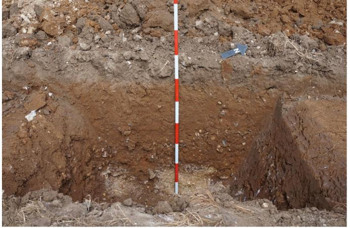
Plate 4: Section of test pit excavated through Head deposit located in south end of Trench 1
